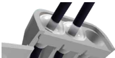
Figure 7. Extra silicone prevents water ingress
